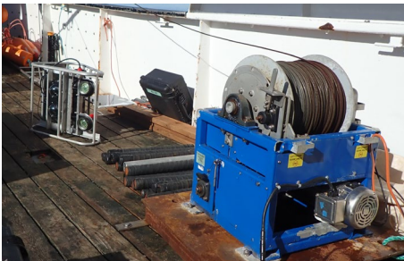
AFSC TowCam: Towable stereo image platform
