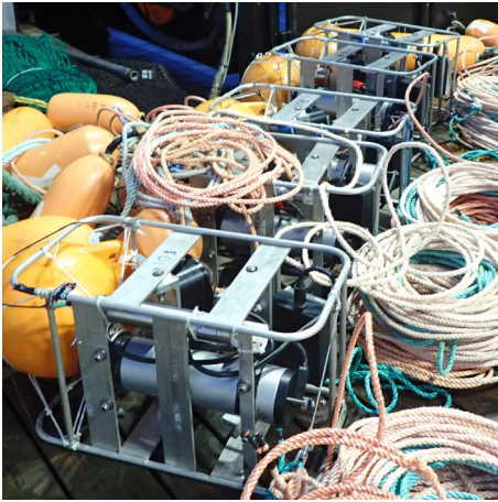
AFSC TrigCams: Stationary paired stereo images
