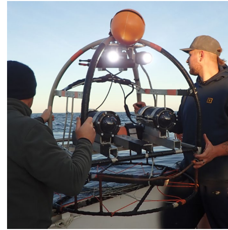
AFSC TrigCams: Stationary paired stereo images
